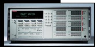
The Model 7002 Switch System is a 10-slot mainframe that supports up to 400 2-pole multiplexer channels or 400 matrix crosspoints. The front panel includes a unique interactive display of channel status for quick programming. Scanning speeds of up to 165 channels per second are possible with the high density switch cards. The wide selection of more than 40 different switch cards makes the 7002 one of the most flexible switching mainframes available.
